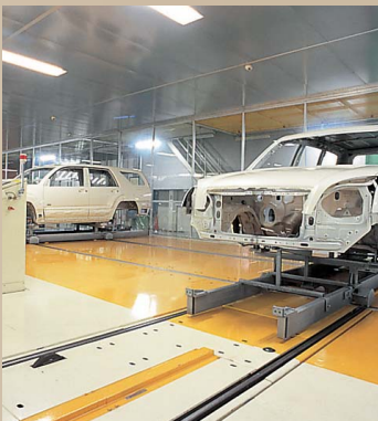
Conveyance System for Automobile Painting Lines
