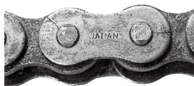
Hydrogen embrittlement cracking
