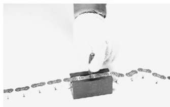
Figure 16: Disconnecting Poly Steel Chain
