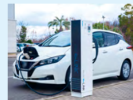
V2X bi-directional EV charging systems (eLink) that contribute to realizing a smart energy society
