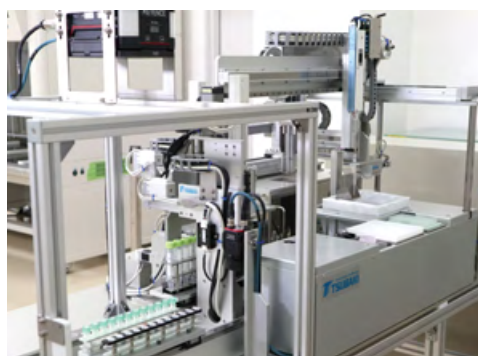
Equipment for automated PCR testing
